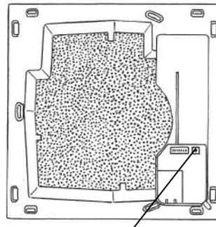
Button for resetting filter monitoring
