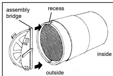
Slide the fan insert into the mounting tube, positioning the mounting bar of the wind pressure protection vertically, connect the power supply, put on the inner cover with the filter frame.
